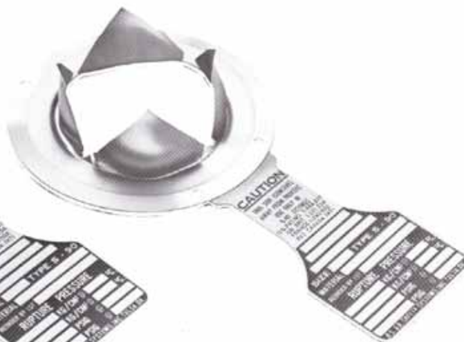
Figure 21: Scored type reverse buckling rupture disk, after rupture.
