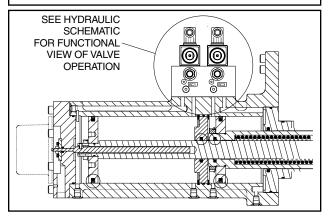
Figure 18. Solenoid Valves And Cylinder
