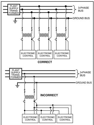
Figure 48. Electronic Control Panel Power Supplies
