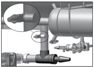
Figure 2. Oil Drain Valve
