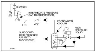
Figure 8. Shell and Coil Economizer System
