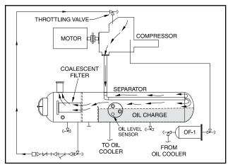
Figure 16. Oil Separation System
