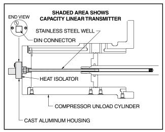
Figure 40. Capacity Linear Transmitter
