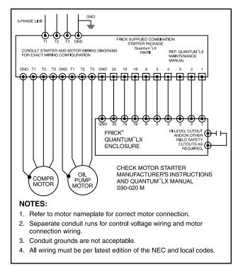
Figure 13. Point-To-Point Wiring Diagram
