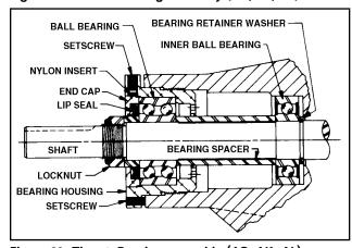
Figure 32. Thrust-Bearing assembly (AS, AK, AL)
