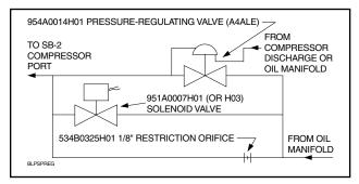
Figure 28. High-Stage SB-2 Oil Supply Line Diagram
