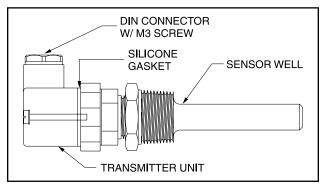
Figure 42. Temperature Transmitter
