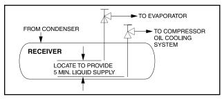
Figure 6. Dual Dip Tube
