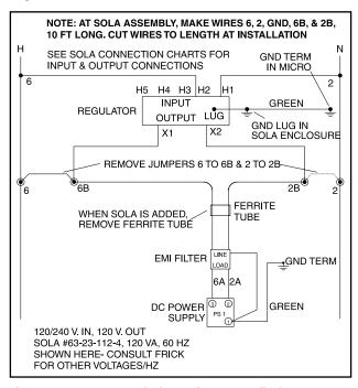
Figure 14. Recommended Regulator Installation
