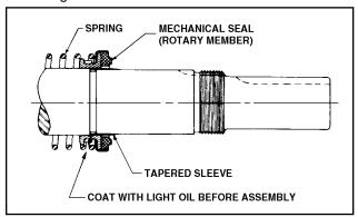
Figure 33. Shaft With Sleeve
