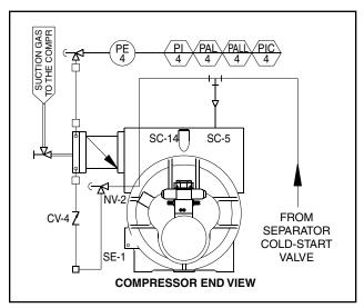
Figure 26. Suction Check Valve Bypass
