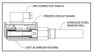
Figure 41. Volume Ratio Control Transmitter
