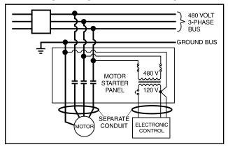
Figure 47. Separation Of Different Voltage Circuits
