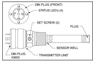
Figure 43. Oil Level Transmitter
