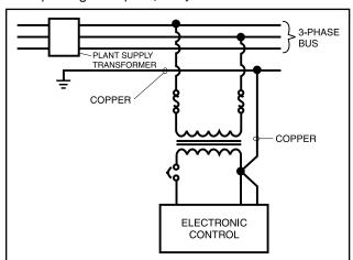
Figure 45. Control Power Ground Circuit
