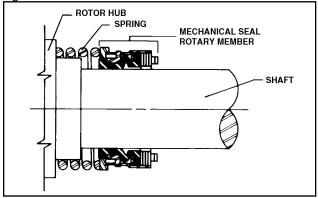
Figure 34. Shaft With Seal Spring
