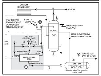
Figure 5. TSOC Piping Arrangement
