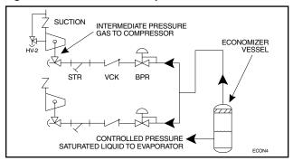
Figure 11. Multiple Compressor Economizer System
