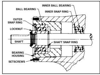
Figure 31. Thrust-Bearing assembly (GG, HJ, HL)
