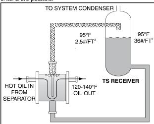
Figure 4. Thermosyphon Receiver System
