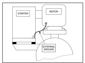
Figure 46. Motor And Starter Grounding
